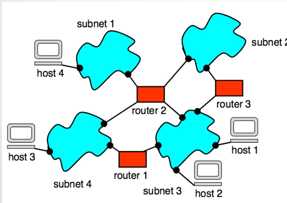
Host: computer connected to the internet, it can be a client or a server at the application level
