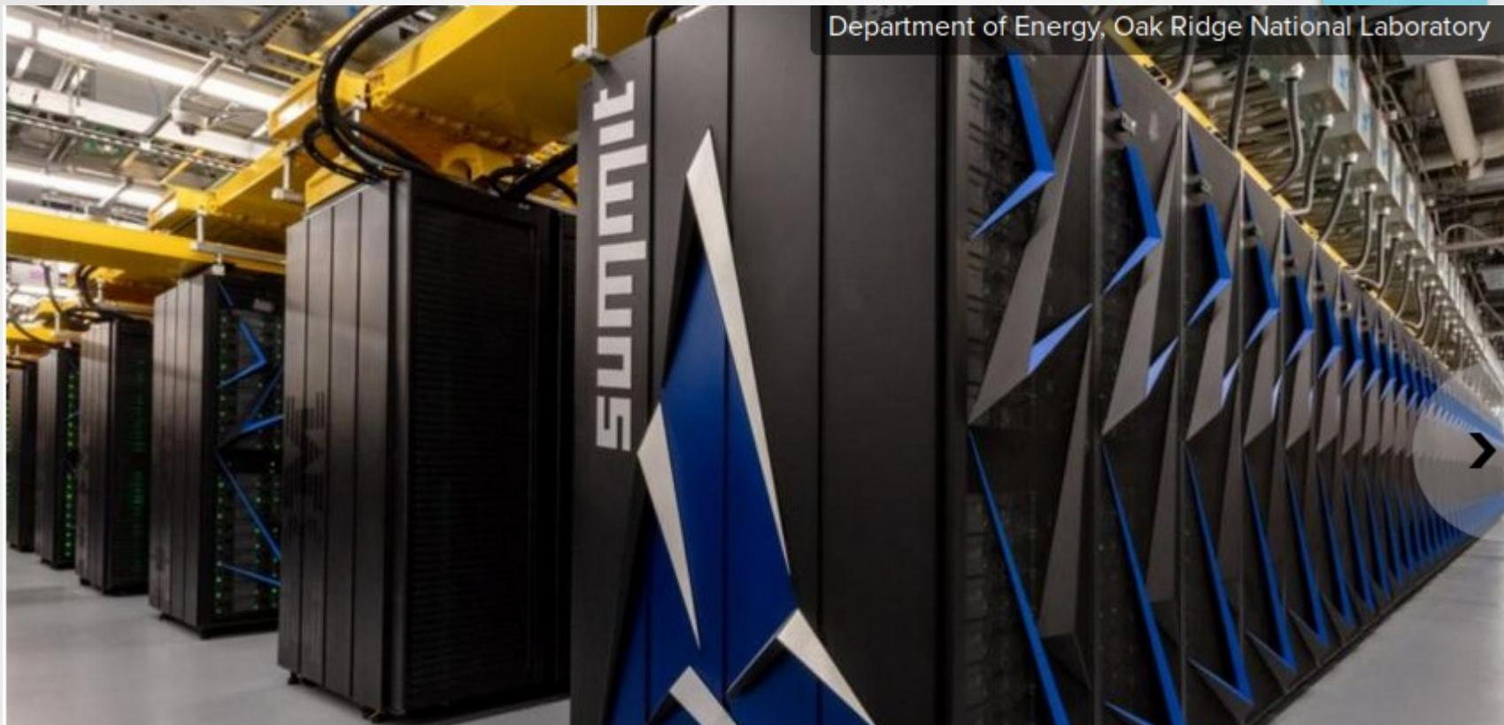
IBM Power System AC922, IBM POWER9 22C 3.07GHz, NVIDIA Volta GV100, Dual-rail Mellanox EDR InfiniBand
